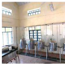
Rice Cooking Machine (Avg. 20 Kgs in ~15 Mins.)
