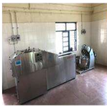
Dough mixing and Chapatti Making Machine (Avg. 500 Chapattis per Hr.)
