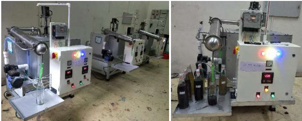
Plastic (PP & PE) and waste oil processing reactors to generate hydrocarbons
